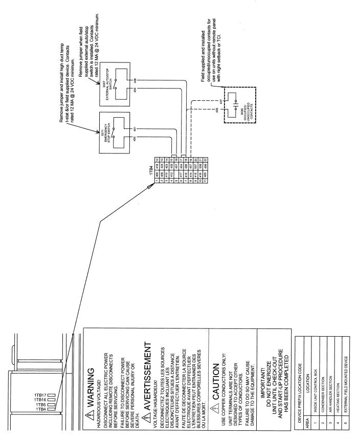
Note: All wiring and components shown dashed to be supplied and installed by the customer in accordance with local electrical codes.
