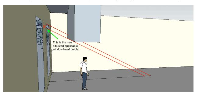
c) With the new adjusted applicable window head height, determine the window surface area SF that can count towards this calculation.
