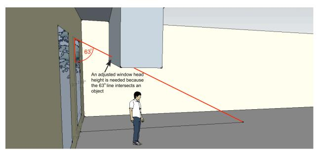
b) Move the 63 degree top line down until it no longer intersects the solid object. The point at which this adjusted line touches the window top will be the adjusted applicable window head height.
