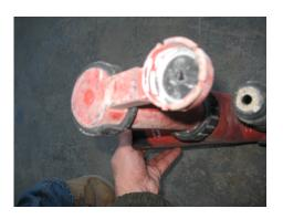
Specialty dust collecting drill used for ceiling drilling to minimize airborne dust.
